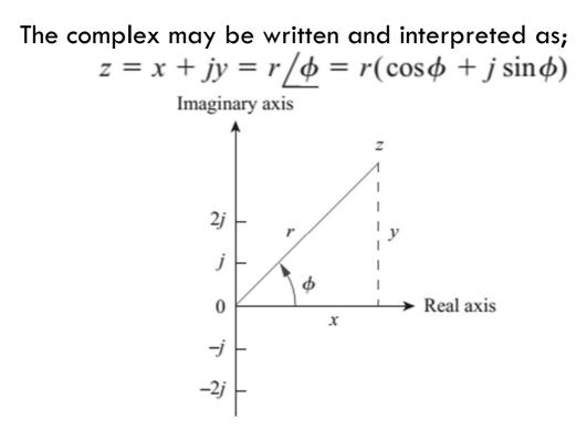
Addition and subtraction of complex numbers are better performed in rectangular form while multiplication and division in polar form.
